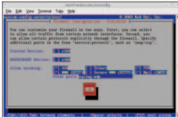
FIGURE ONE: Screen dumps from system-config-securitylevel , used to create a hole for incoming syslogd messages on the master node/server
